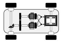
With our Hardware-in-the-Loop (HiL) test infrastructure for dual-drive propulsion systems (for example in electric vehicles) you can assess the performance of dual-drive control strategies, virtual sensing and power flow management systems in terms of operational range and energy efficiency. This both at a real-time machine-level
